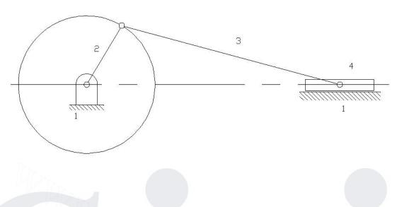
In the above given Slider crank mechanism, link 2 rotates relative to link 1 and constitutes a revolute or turning pair. Similarly, links 2, 3 and 3, 4 constitute turning pairs. Link 4 Slider reciprocates relative to link 1 and its a sliding pair.
