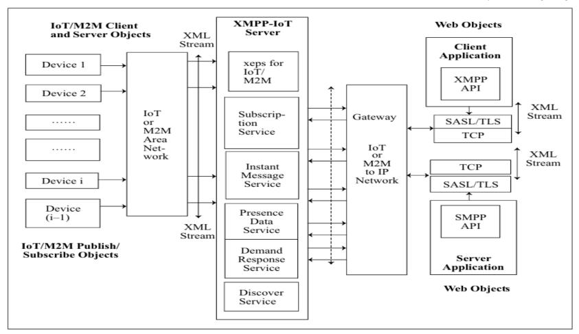
Use of XMPP and XMPP extension protocols for connected devices and web objects for the messaging, presence notifications, responses on demand and service discoveries using XML streams
