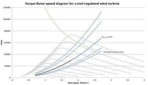
where the black line represents the initial section of the operating strategy for a variable speed stall- regulated wind turbine. Ideally, we would want to stay on the maximum efficiency curve until ratedpower is hit. However, as the rotor speed increases, the noise levels increase. To counter this, the rotor speed is not allowed to increase above a certain value. This is illustrated in the figure below:
