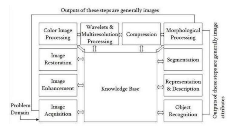
**Fundamental steps and Components in digital image processing** / 19EC513/ IMAGE PROCESSING AND COMPUTER VISION /K.SANGEETHA/ AP/ECE/SNSCE
