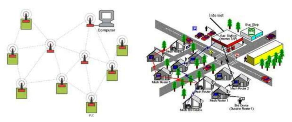
• In a wireless mesh network, multiple nodes cooperate to relay a message to its destination. The mesh topology enhances the overall reliability of the network, which is particularly important when operating in harsh industrial environments.
