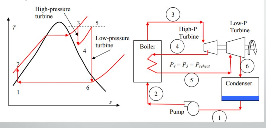
The total heat input and total turbine work output for a reheat cycle become:
