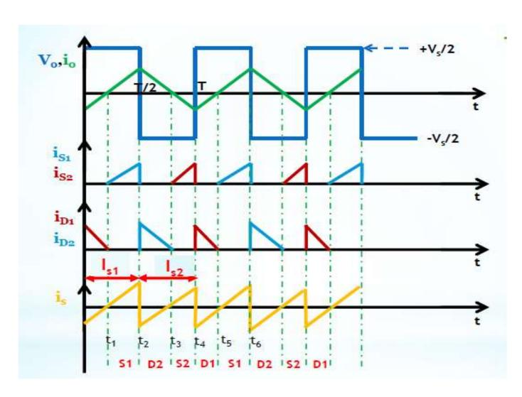
$$V_o(rms) = \frac{1}{T_0/2} \int_0^{T_0/2} \frac{V_s^2}{4} dt = \frac{V_s}{2}$$
