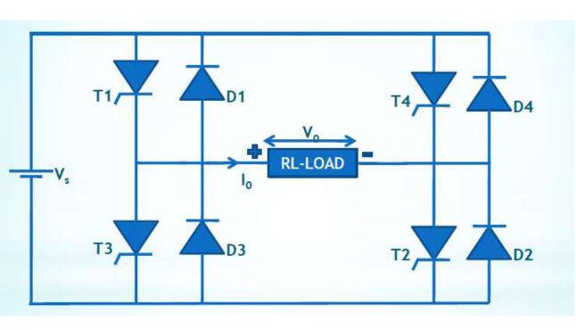
**MODE 1**: T1, T2 ON, SOURCE DELIVERING POWER TO LOAD – Vo +ve, lo +ve.
