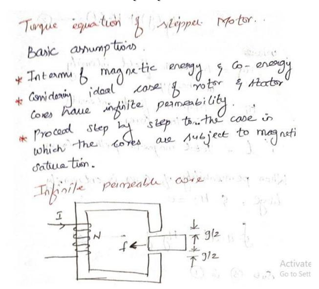
a coverent I, is blowing through the will go I twoens to yield the magnetic blux, for if is acting on ioun piece in the x-direction.
