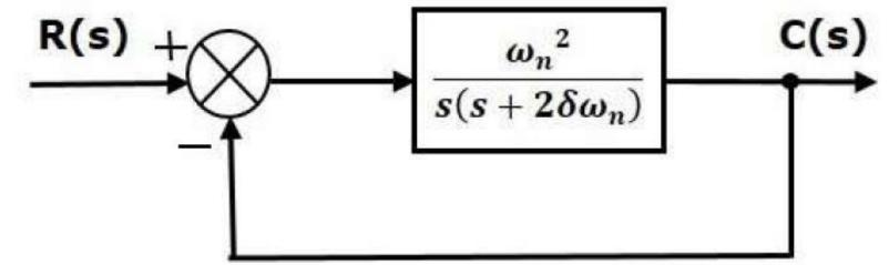
We know that the transfer function of the closed loop control system having unity negative feedback as
