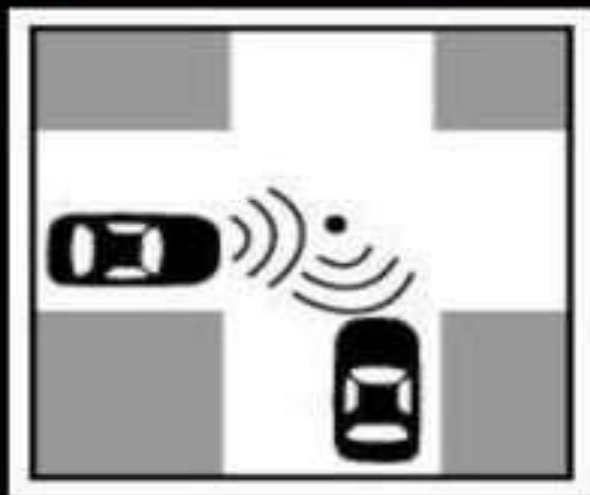
Intersection Collision Warning
