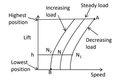
The maximum speed at which the governor will rotate is  $N_A$  when the sleeve is in the highest position and has a tendency to ascend and minimum speed is  $N_B$  when the sleeve is at the lowest position and has a tendency to descend.
