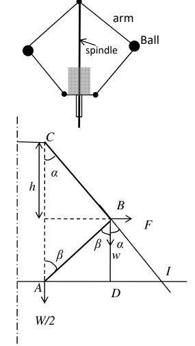
So, it would be observed that the *h* for a given percentage change in speed is increased in the ratio (W+w)/w due to the dead weight.
