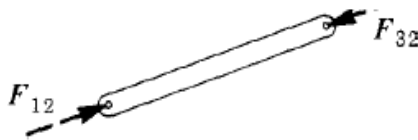
Figure 5.1(D) Free-body diagram of a single link
