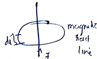
→ The line integral of magnetic field intensity  $\vec{H}$  around any closed path is equal to the total current 'I' enclosed by the path.
