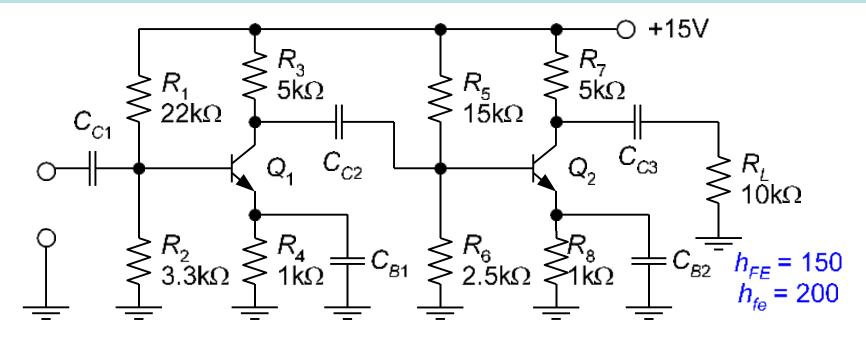
$$Z_{in(base)} = (h_{fe} + 1)r'_{e} = 201 \times 17.4 = 3.497 \text{k}\Omega$$
