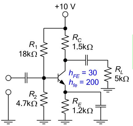
$$V_{th} = V_{CC} \frac{R_2}{R_1 + R_2} = 10V \frac{4.7k\Omega}{22.7k\Omega}$$
