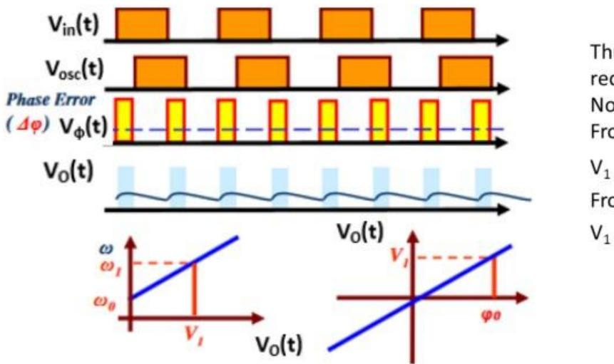
Thus, a high loop gain K<sub>p</sub>K<sub>o</sub> is beneficial for reducing phase errors. Note:
