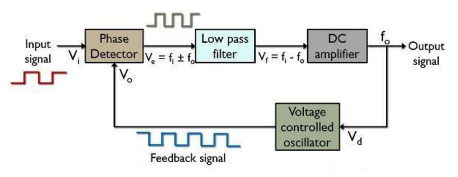
The basic PLL block diagram consists of three components connected in a feedback loop :
