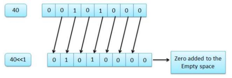
× BITWISE OPERATORS << Shift Left **BINARY FORM** SYNTAX VALUE x = 7;00000111 14 x=x<<1;00001110 112 x = x < < 3; 01110000 192 x=x<<2;11000000
