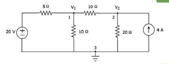
In the above figure,  $V_1$  is the voltage from node 1 with respect to ground and  $V_2$  is the voltage from node 2 with respect to ground.
