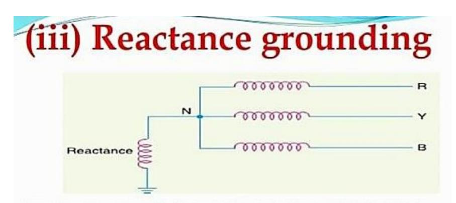
In this system, a reactance is inserted between the neutral and ground
