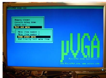
Embedded system text user interface using MicroVGA<sup>[nb 1]</sup>
