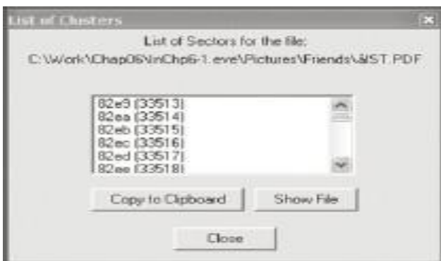
Figure 5-9 Chained sectors associated with clusters as a result of increasing file size Courtesy of Technology Pathways, LLC
