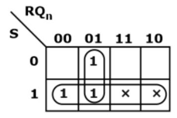
The characteristic equation of SR flip-flop from the above K-map is
