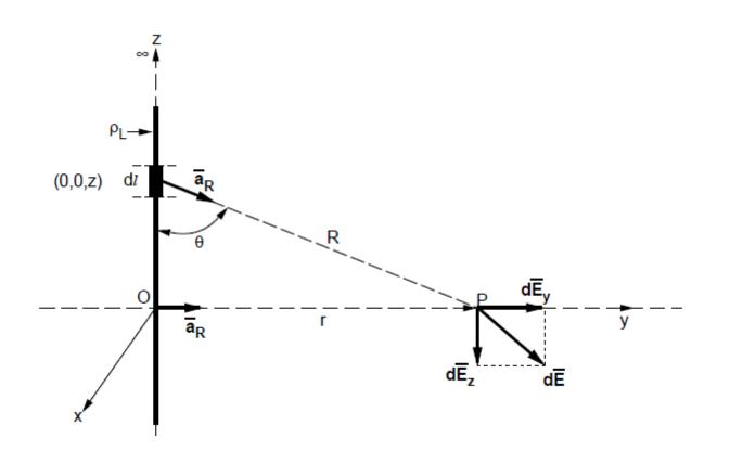
ELECTROMAGNETIC FIELDS AND WAVES/23ECT202/ Dr. A. Vaniprabha Electric Field Due to an Line Charge
