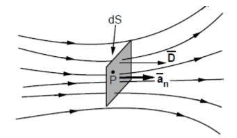
$d\psi$  = Total flux lines crossing normal through the differential area dS
