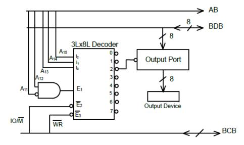
The interfacing circuit makes use of 3 Line to 8 Line decoder having 3 enable lines  $E_1$ ,  $\overline{E_2}$ ,  $\overline{E_3}$ . The address of the device is
