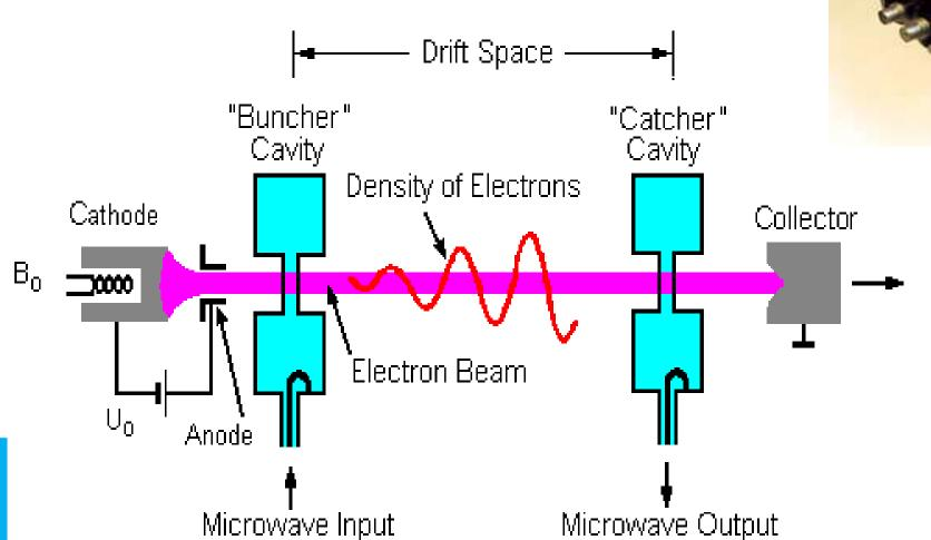
Two cavity klystron amplifier / 19EC602/ Microwave and Optical Engineering/Mrs.D.Vishnu Priya /ECE/SNSCE
