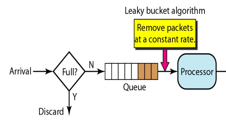
A leaky bucket algorithm shapes bursty traffic into fixed-rate traffic by averaging the data rate. It may drop the packets if the bucket is full.
