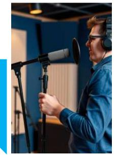
Place the microphone as close to the sound source as possible, maintaining a consistent distance and angle.
