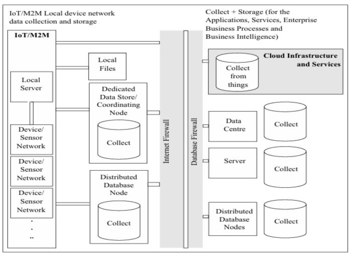
Devices or sensors network data collection at a device local-server, local files, dedicated data store, at a coordinating node, a local node of a distributed DBMS, Internet-connected server of data centre, server or distributed database nodes or a cloud infrastructure
