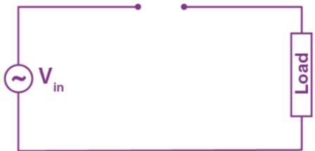
When a diode is reverse biased, it acts as an open switch. Since no current can flow to the load, the output voltage is equal to zero.
