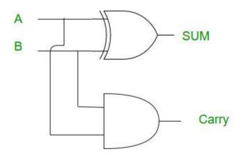
**Note:** Half adder has only two inputs and there is no provision to add a carry coming from the lower order bits when multi addition is performed.
