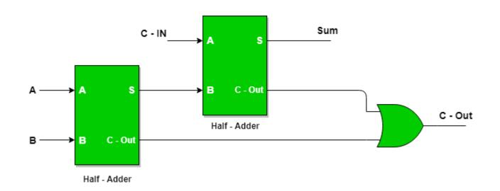
With this logic circuit, two bits can be added together, taking a carry from the next lower order of magnitude, and sending a carry to the next higher order of magnitude.
