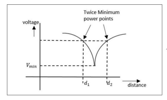
Now, the VSWR can be calculated by a relation, given as  $VSWR = \lambda g \pi (d2 - d1)$ Where,  $\lambda g$  is the guided wavelength  $\lambda g = \lambda 0 / 1 - (\lambda 0 \lambda c) 2$ Where,  $\lambda 0 = c/f$
