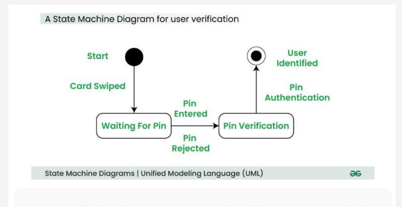
The State Machine Diagram above shows the different states in which the verification sub-system or class exist for a particular system.
