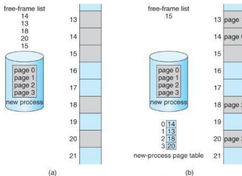
Figure 8.13 - Free frames (a) before allocation and (b) after allocation
