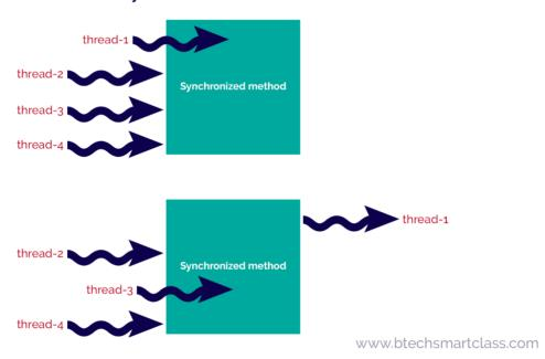
In the above image, initially the thread-1 is accessing the synchronized method and other threads (thread-2, thread-3, and thread-4) are waiting for the resource (synchronized method). When thread-1 completes it task, then one of the threads that are waiting is allocated with the synchronized method, in the above it is thread-3.
