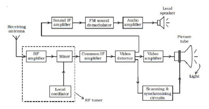
Fig Elementary block diagram of a monochrome TV receiver
