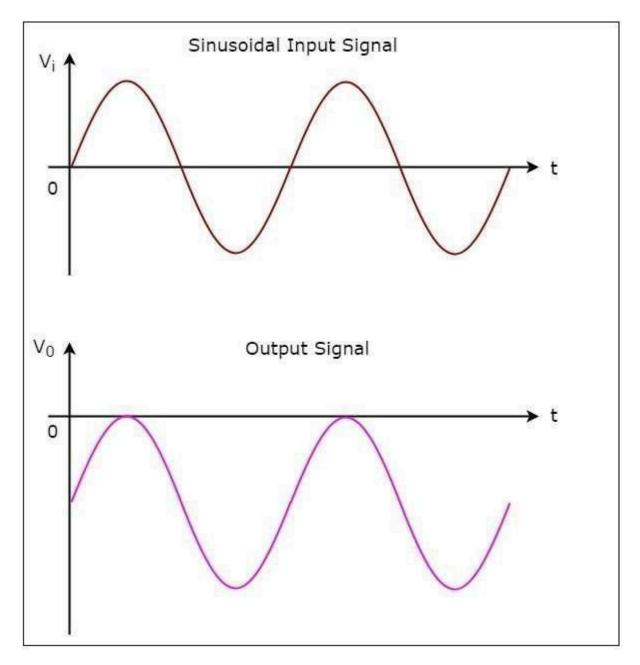
We can observe from the output that the negative clamper shifts the applied input waveform **vertically downward** at the output. The amount of shifting will depend on the value of DC reference voltage.
