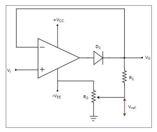
In the above circuit, a sinusoidal voltage signal Vi is applied to the non-inverting terminal of the op-amp. The value of the reference voltage *Vref* can be chosen by varying the resistor R2.
