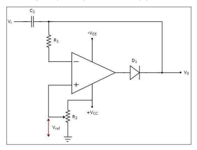
In the above circuit, a **sinusoidal voltage signal**, Vi is applied to the inverting terminal of op-amp through a network that consists of a capacitor C1 and a resistor R1. That means, AC voltage signal is applied to the inverting terminal of the op-amp.
