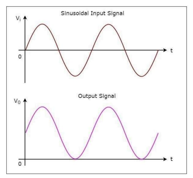
From the figure above, you can observe that the positive clamper shifts the applied input waveform **vertically upward** at the output. The amount of shift will depend on the value of the DC reference voltage.
