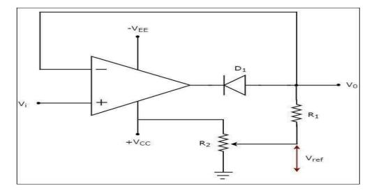
In the circuit shown above, a sinusoidal voltage signal VtVt is applied to the non-inverting terminal of the op-amp. The value of the reference voltage VrefVref can be chosen by varying the resistor R2R2.
