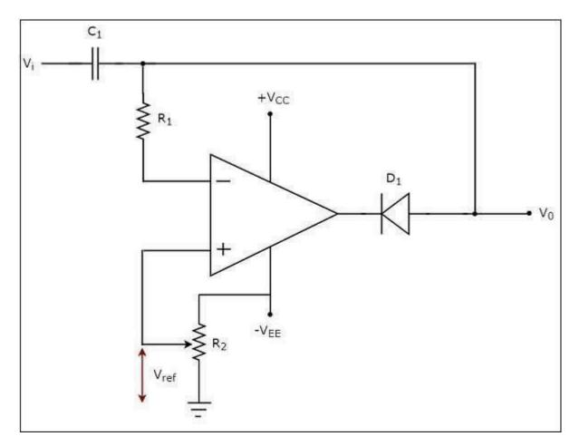
In the above circuit, a **sinusoidal voltage signal** Vi*Vi* is applied to the inverting terminal of the op-amp through a network that consists of a capacitor  $C_1$  and resistor R1. That means, AC voltage signal is applied to the inverting terminal of the op-amp.
