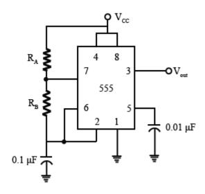
The output is produced with frequency of 2 kHz and duty cycle of 75 %, then find the value of resistance  $R_B$  and  $R_A$  are respectively
